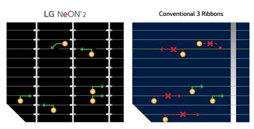
Multiple electrical paths maintained by wires
